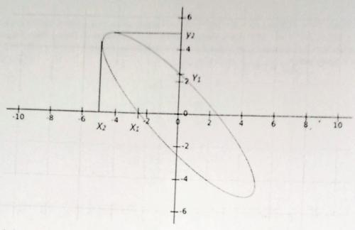
As we studied above it Clear that when the angle is in the range of  $0^{\circ} < \emptyset < 90^{\circ}$  or  $270^{\circ} < \emptyset < 360^{\circ}$ , the Lissajous quadrant:
