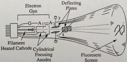
When both pairs of the deflection plates (horizontal deflection plates and vertical deflection plates) of CRO (Cathode Ray Oscilloscope) are connected to two sinusoidal voltages, the patterns appear at CRO screen are called the Lissajous pattern.
