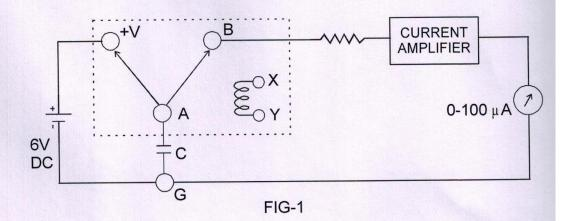
The components within the dotted box constitutes the reed switch. It is a changeover switch that charges the capacitor C through contact A and then discharges C through the electronic micrometer via the contact B. The charge discharge rate is double the frequency of the voltage applied to X, Y terminals of the coil of the reed switch. Since the mains frequency is 50 Hz, we should use a value f = 100 Hz in equation (2)
